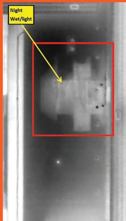
Moisture survey using a drone nighttime infrared scan
