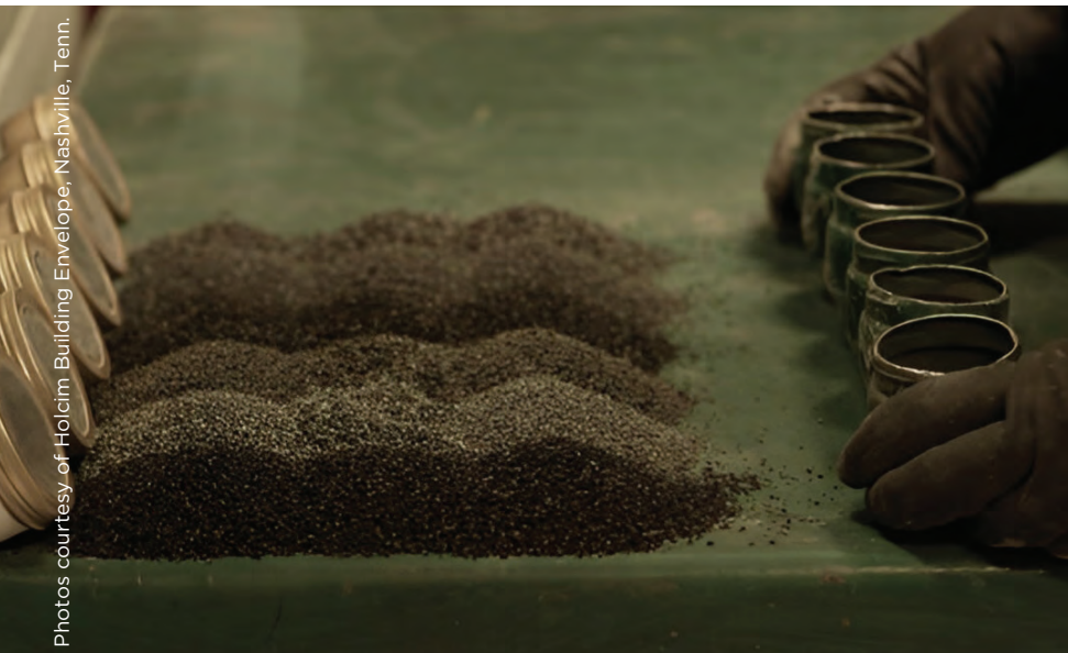
Photos courtesy of Holcim Building Envelope, Nashville, Tenn. Malarkey Roofing Products has recovered millions of pounds of granules from the manufacturing process.
